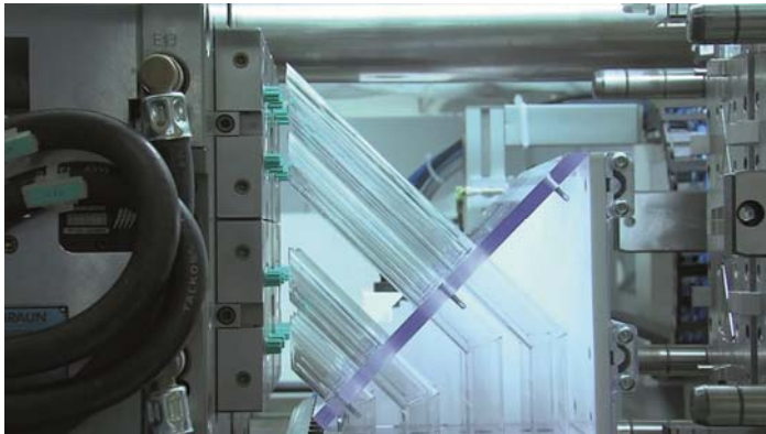
Every cavity is individually intercepted by a Braunform patented handling. (© Braunform GmbH)
