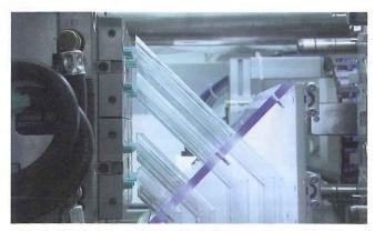
TELC is a tamper-proof closure system for prefillable syringes. During clean-room production, each cavity is served individually by a patented handling system (figures: Gerresheimer Bünde, Braunform)
