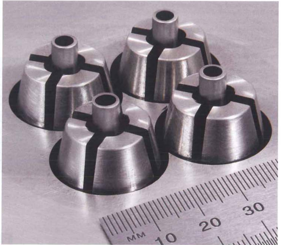
<< Expandable cavities allow for very tight cavity spacing compared to slides, allowing for more cavities per mould or a smaller mould and press. >>
