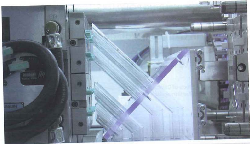
<< This Braunform two component (twin shot) mould manages a temperature gradient between a polycarbonate shot of 100°C and that of a TPE at 40°C. >>
